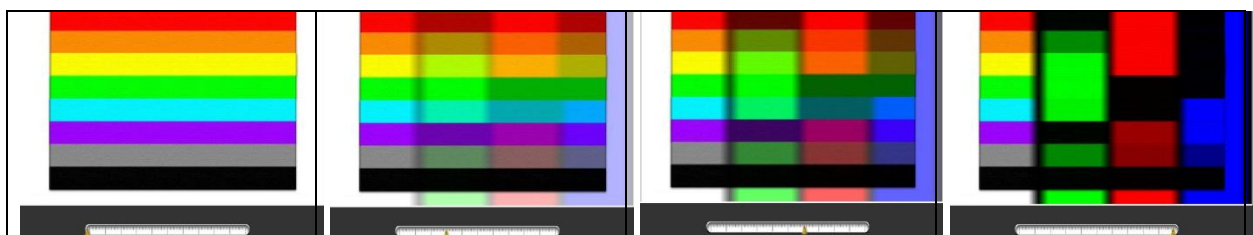
Figure 5: This sequence shows what happens if you illuminate the horizontal 8 color bars on the left with more and more monochromatic light in 3 vertical bars with red, green and blue. The image on the right only shows those bars that reflect some of this monochromatic light, all the others turn black. Interactive graphic can be found at (6)
