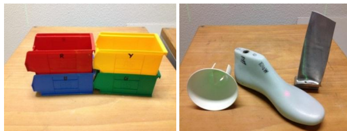
Figure 6: Scene A (left) was used to test the performance of different colors, scene B has typical difficult surfaces for white light scanners. Note the red dot on the shoe-last is a spot of a laser pointer that is blurred through the translucent surface
