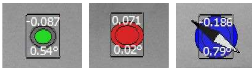
Figure 9: A color code marks each fastener for easy interpretation of measurement results
