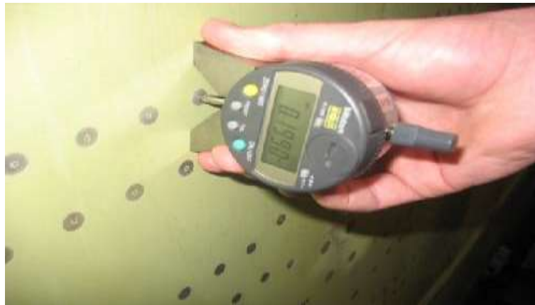
Figure 6: A manual dial gage is used to measure fastener flushness
