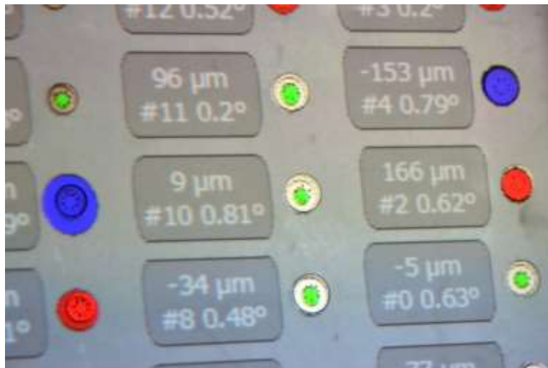
Figure 3: Augmented Overlay for fastener flushness measurement
