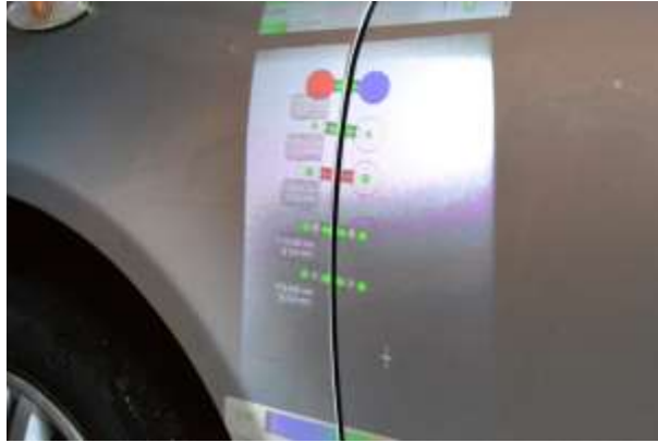
Figure 15: gapCHECK is able to measure gap and flush deviation
