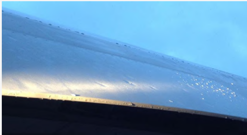
Hail Damage (Image source: easyJet)
