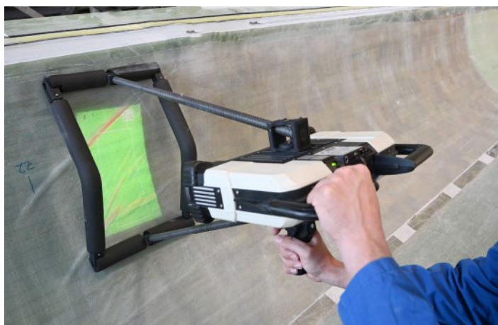
RESULTS ARE PROJECTED DIRECTLY ON TO THE BLADE
