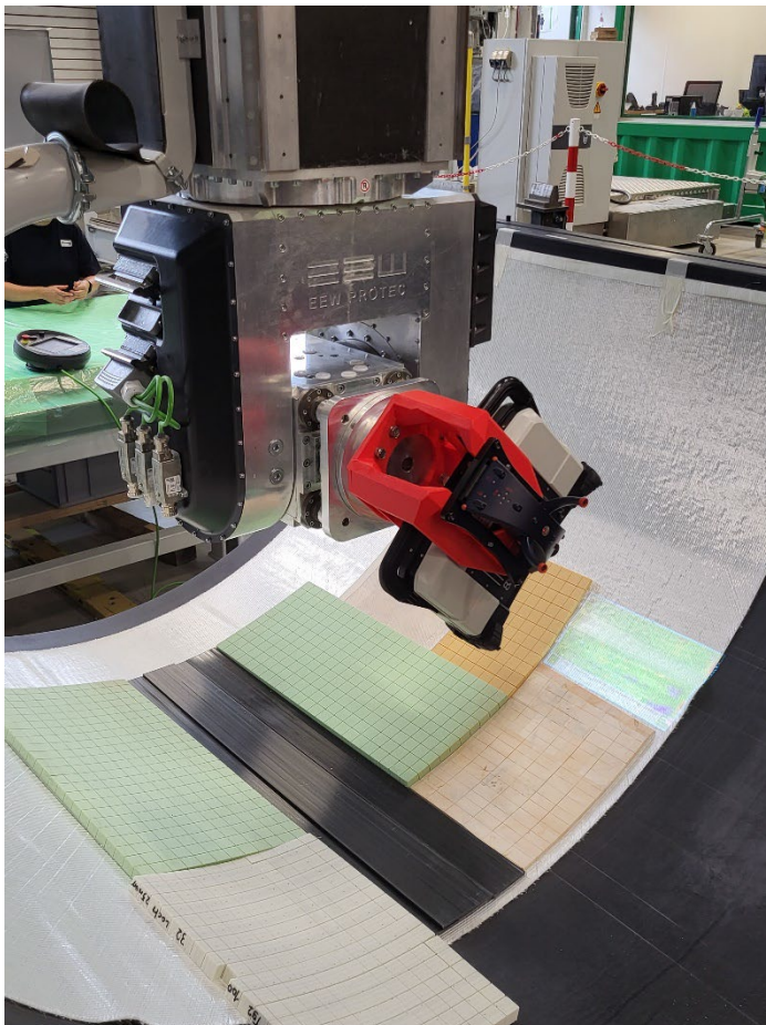
Figure 1: 8tree scanner integrated in experimental blade manufacturing environment at Fraunhofer IWES.
